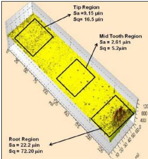
Figure 24. Surface Roughness and Topography of TTO Pinion After 33.5 hrs of Testing
