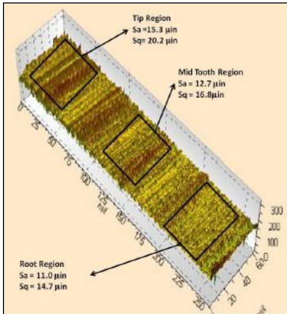
**Figure 28. Surface Roughness and Topography of TTO Gear After 33.5 hrs of Testing**
