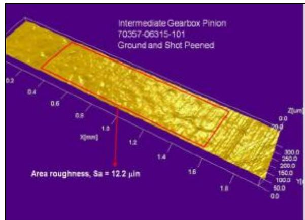
Figure 26. Surface Roughness and Topography of New Production IGB Pinion
