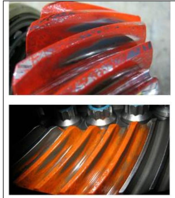
**Figure 17. Contact Pattern Achieve During Assembly with Pinion C518-00159**
