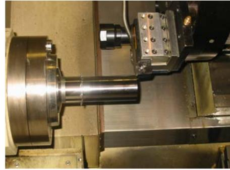
**Fig.4.** Experimental set-up of Ti-6Al-4V turning test
